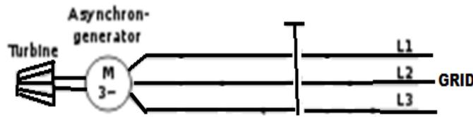
Schematic diagram of a standalone grid-excited induction generator
