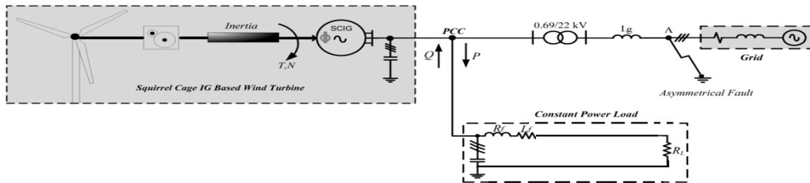
block diagram of GCIG with fault in grid side
